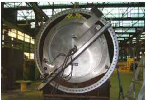
▼ Wind tower machining with WP4600.
