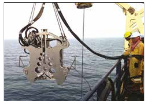
▲ MDWS Diamond Wire Saw lowered into sea.
